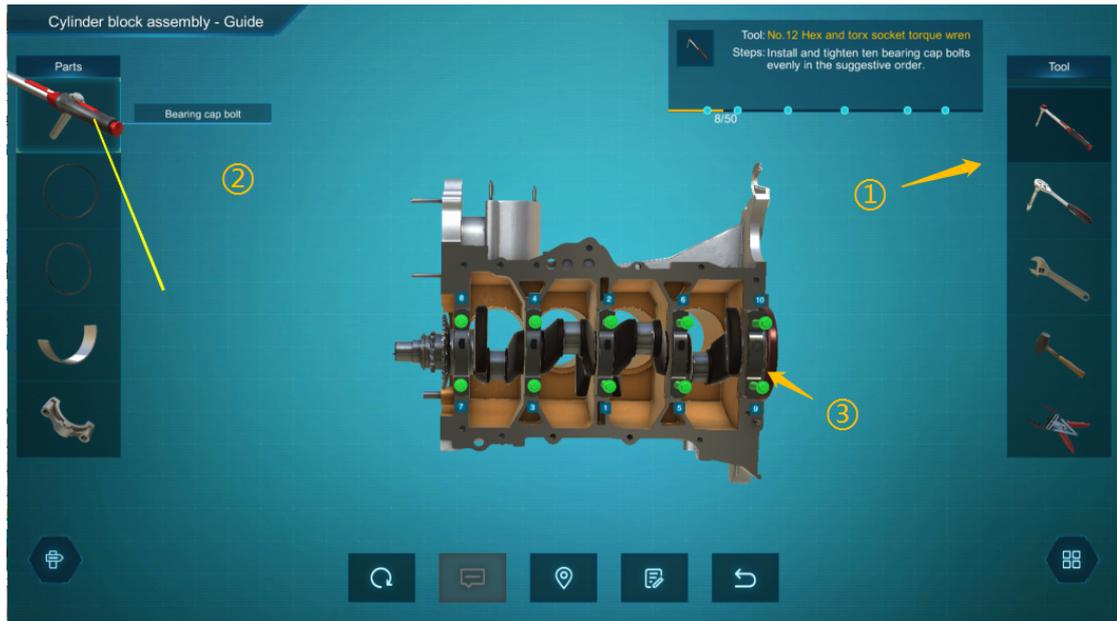
Figure 4-2-7-3 Operating instructions on installing lubricating parts
