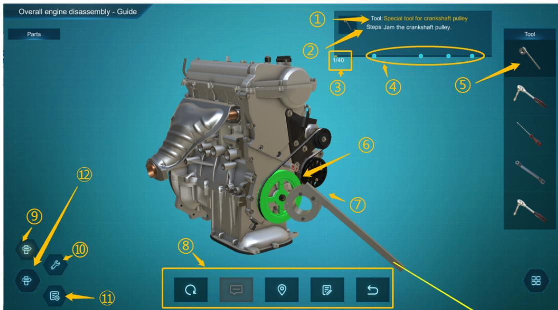
Figure 4-2-6-2 Operation of engine disassembly
