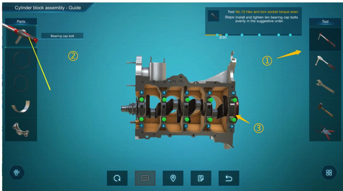
Figure 4-2-7-2 Operating instructions on installing a bolt/nut
