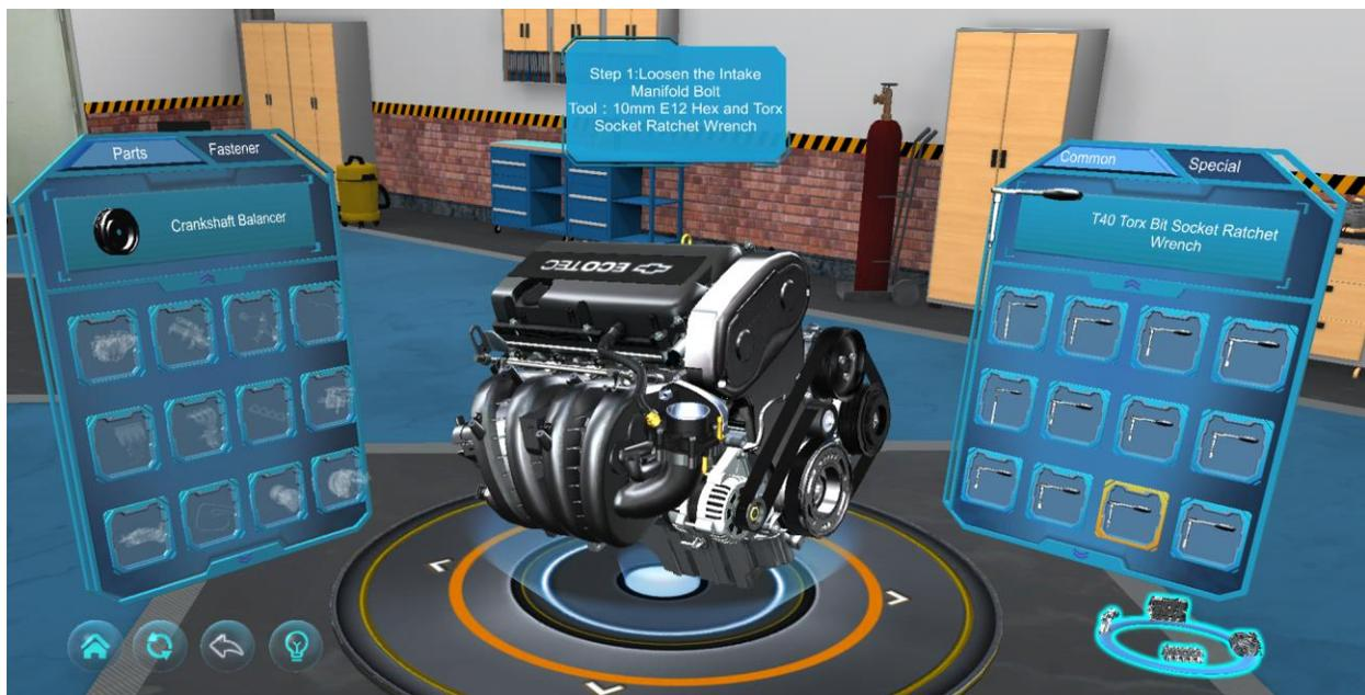
The disassembly interface layout is as shown in the picture above. On the left, the parts rack is composed of components and fasteners. When the disassembly is completed, all parts will be returned to the rack automatically. The middle panel is a prompt box which shows the operating details of the current step. On the right, the tool rack contains
