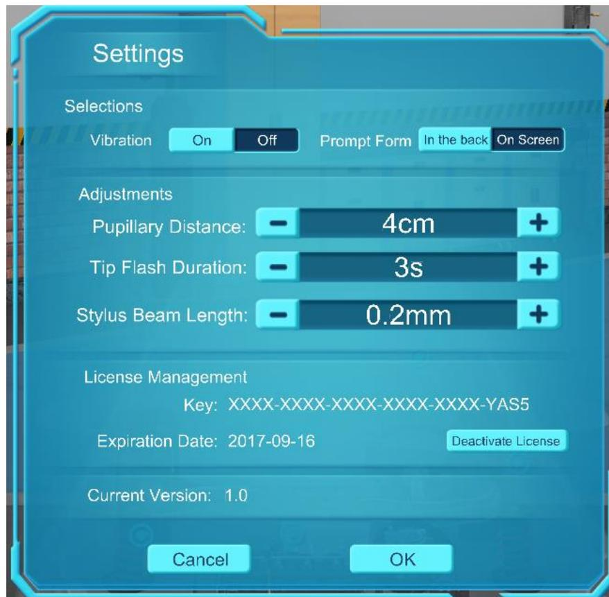
Users can set their own operating preferences for stylus vibration, the position of the prompt panel, pupillary distance, tip flash duration, and stylus beam length.
