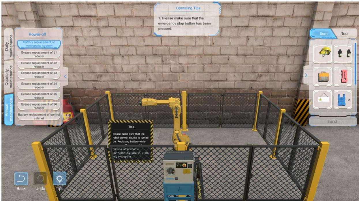
There are eight modules in the navigation bar: Battery replacement of mechanical system, Grease replacement of J1 reducer, Grease replacement of J2 reducer, Grease replacement of J3 reducer, Grease replacement of J4 reducer, Grease replacement of J5 reducer, Grease replacement of J6 reducer, and Battery replacement of control cabinet. Select one module to show the corresponding scenario.
