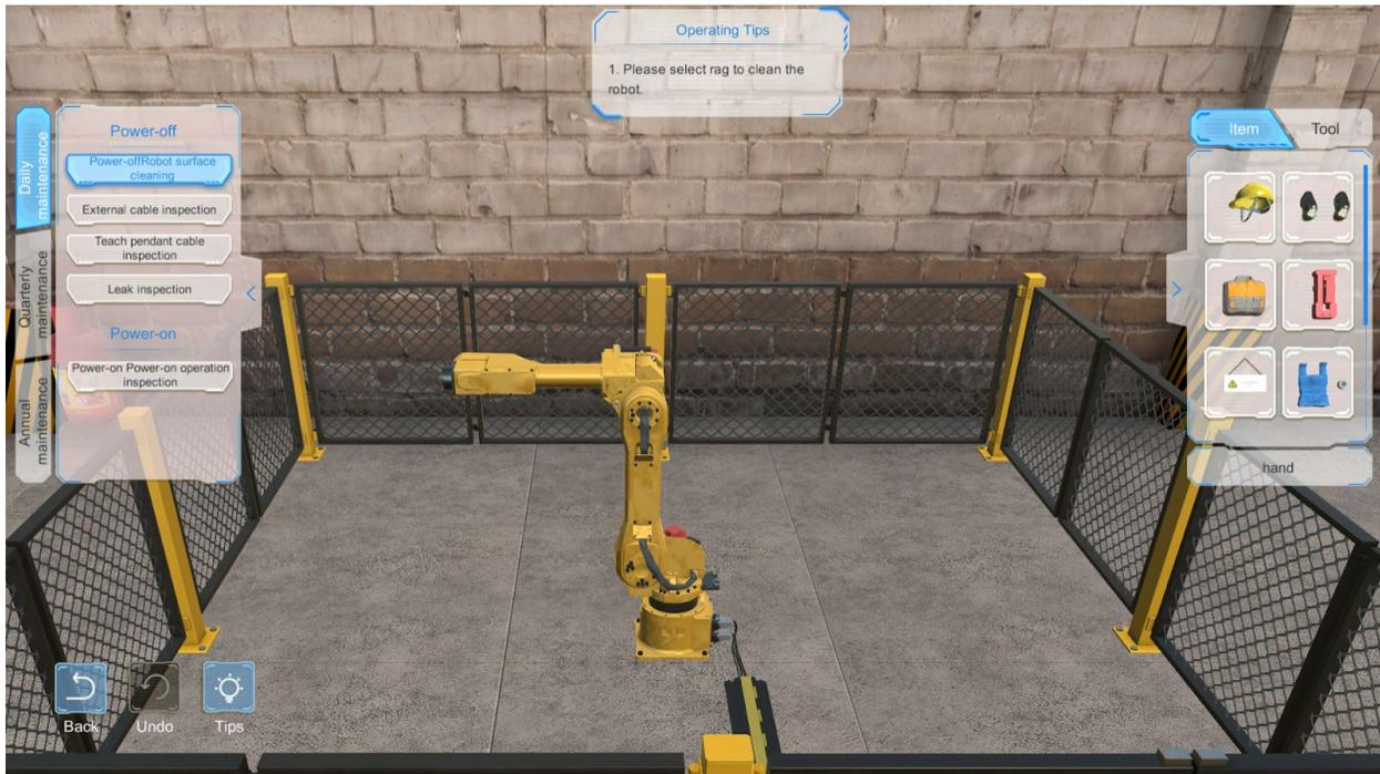
There are five modules in the navigation bar: Robot surface cleaning, External cable inspection, Teach pendant cable inspection, Leak inspection, and Power-on operation inspection. Select one module to show the corresponding scenario.
