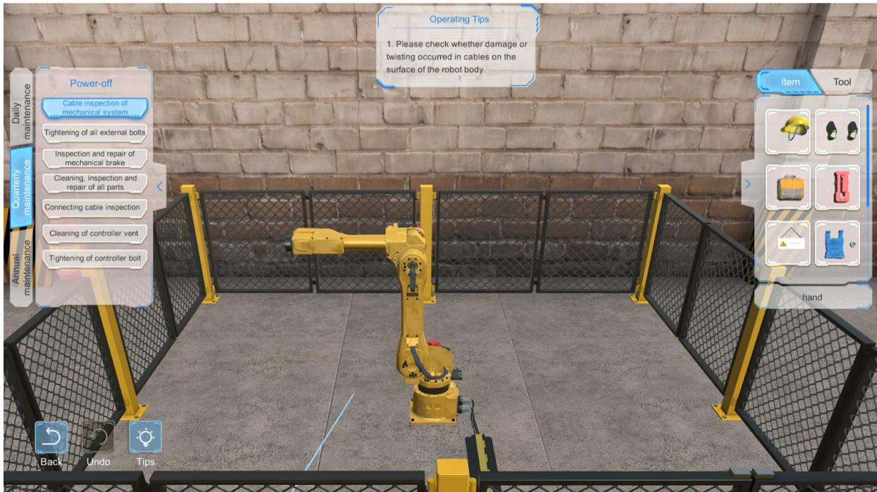
There are seven modules in the navigation bar: Cable inspection of mechanical system, Tightening of all external bolts, Inspection and repair of mechanical brake, Cleaning, inspection and repair of all parts, Connecting cable inspection, Cleaning of controller vent, and Tightening of controller bolt. Select one module to show the corresponding scenario.
