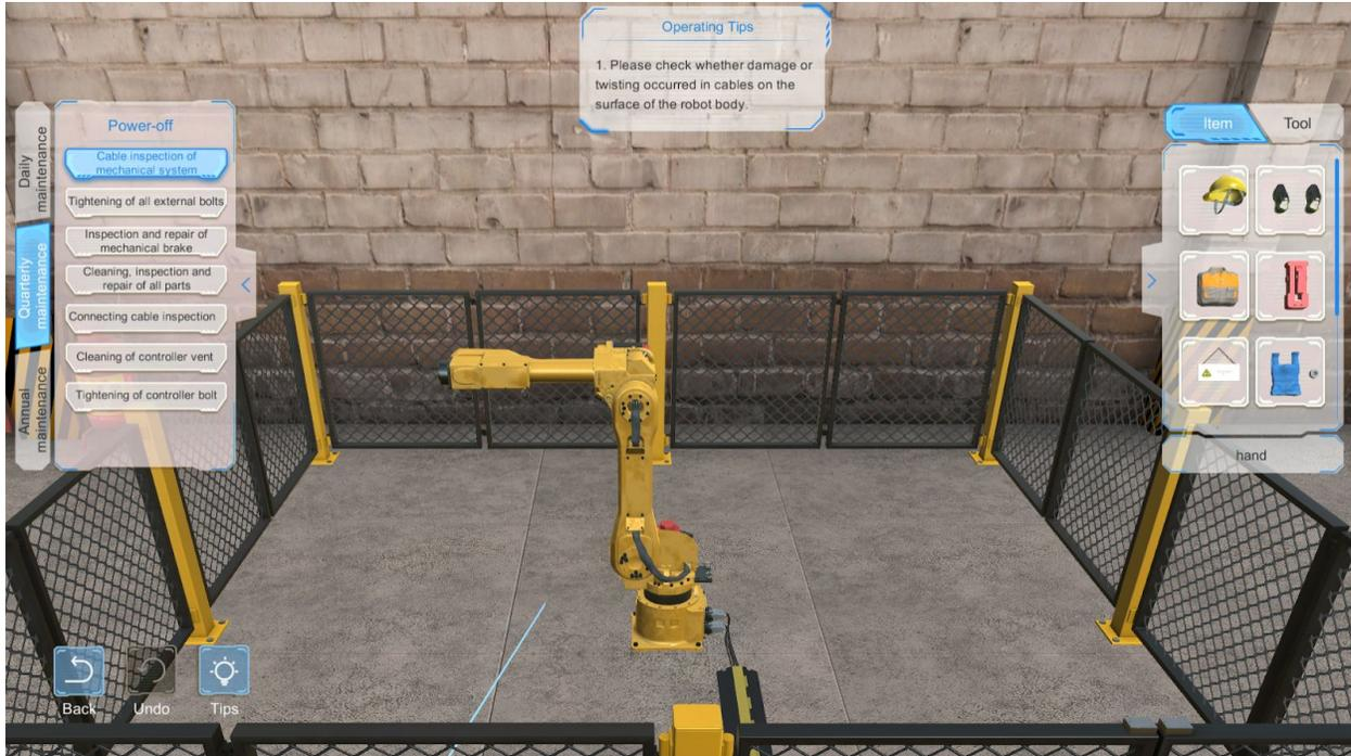
Click on the “Tightening of all external bolts” in the navigation bar to show the corresponding scenario.
